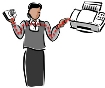
Fig. 2. A conceptual example of “Touch-and-Play” [Park et al. 2006a, 2006b]: a user can print a desired photo stored in a digital camera by touching a printer while holding the camera.
