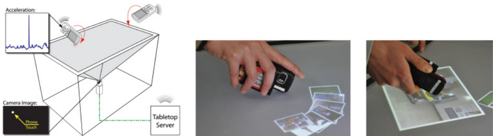
Fig. 9. “PhoneTouch” [Schmidt et al. 2010]: (Left) An illustration showing how the system detects phone tapping events. (Center) A user drops a collection of photos on a surface. (Right) A user picks up a photo by tapping on it. (Reprinted with permission of Dominik Schmidt.)
