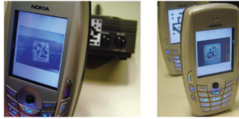
Fig. 3. Examples of “Seeing-Is-Believing” (SiB) [McCune et al. 2005, 2009]. A phone running SiB scans the barcode of a target device to capture its cryptographic information. (Left) Static visual barcode. (Right) Dynamic visual barcode. (Reprinted with permission of Jonathan McCune.)
