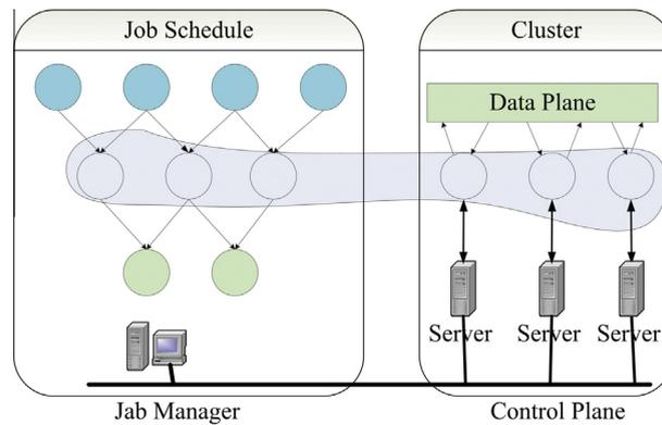
Fig. 9. Dryad architecture.
