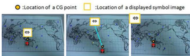
Fig. 6. Three display methods. On the left is AR Annotation wherein a label is placed near the relevant part of the map. The middle and right are control scenarios wherein a label is displayed randomly on the map with a connecting line, and a label is displayed consistently at the top left of the HMD screen without a connecting line, respectively [35].
