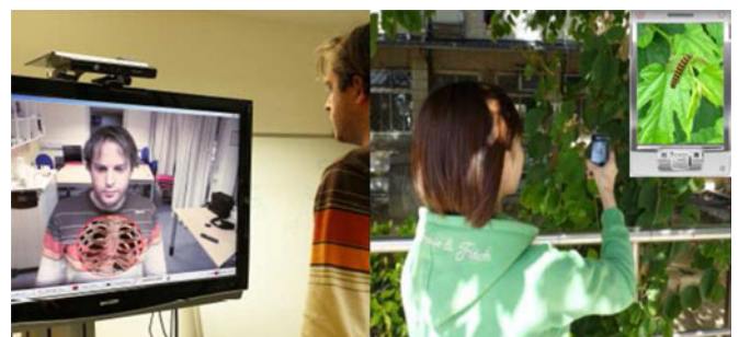
Fig. 3. Mirror metaphor (left) where the real environment used is behind the user [14]; and Glasses Metaphor (right) where the real environment used is in front of the user [104].
