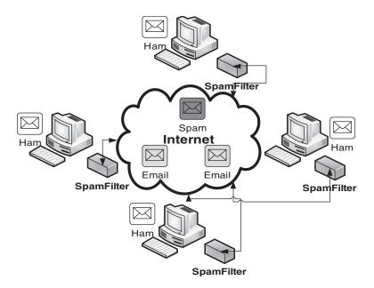
Fig. 1. Peer-to-peer computing for spam filtering.
