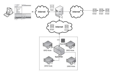
Fig. 2. Grid computing for spam filtering.
