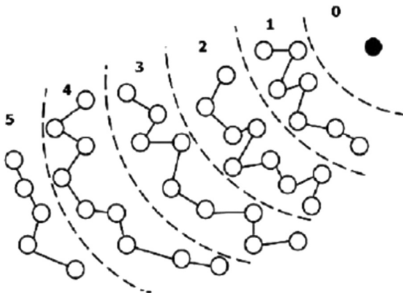
Fig. 7. Constructing the chains in a tracked WSN by CCS (redrawn from Jung et al., 2007).
