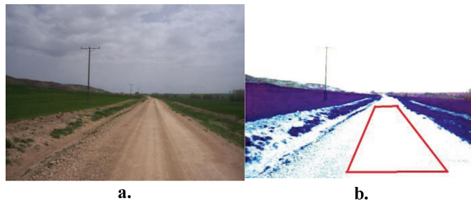
Fig. 7. Texture analysis: (a) Original image; (b) refined image (white fields point to the road, blue fields point outside).
