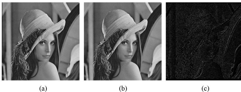
Fig. 12. (a) Standard Lena Image. (b) Watermarked Image using Thodi et al.'s scheme [92] with PSNR = 37.01 dB, and embedding capacity of 0.4 bpp. (c) Enhanced difference of (a) and (b).
