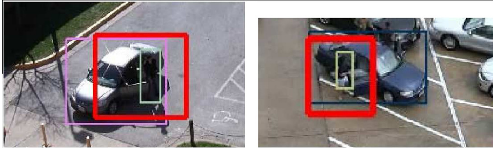
Fig. 27. Examples of ground truth from VIRAT database where both the person and vehicle bounding boxes are plot in different colours, and the event boxes are marked by thick red box.
