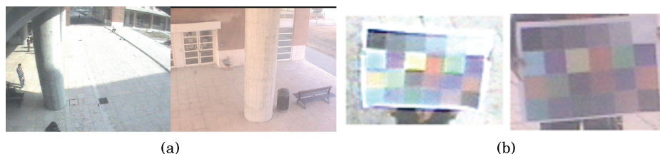
Fig. 4. A common problem of multicamera systems: (a) different views have different colors; (b) patterns used for the color calibration.
