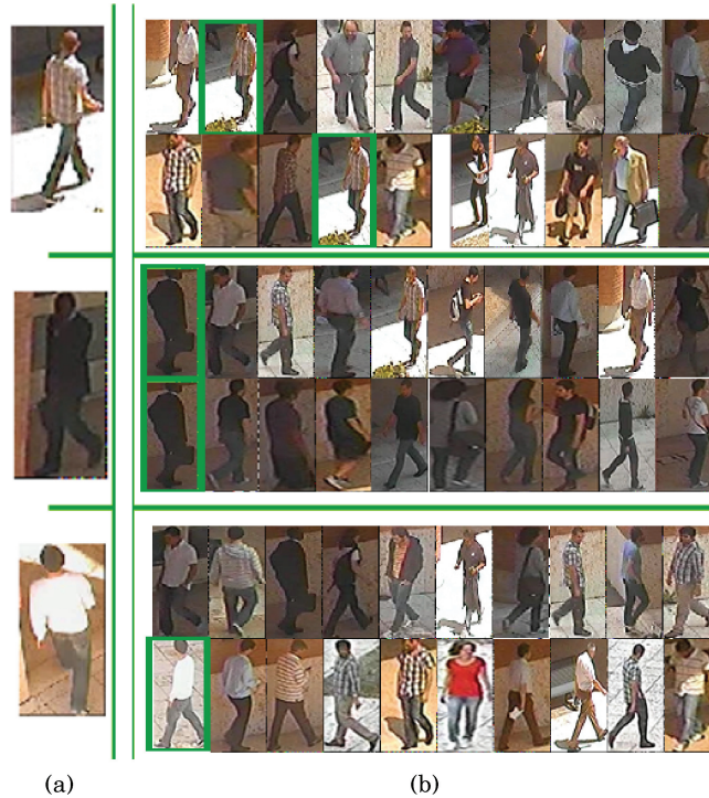
Fig. 9. Three example queries using the 3DPes dataset. (a) Probe image (for Sarc3D this is just one of the images used for the model creation). (b) The top 10 results (sorted left to right) using SDALF (top) and Sarc3D results. The correct match is highlighted in green.
